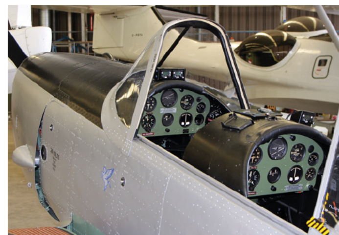
ABOVE: The subject of a long-term restoration at Duxford, which concluded with a maiden flight in December 2015, the Loweth Flying Group's WK522/G-BCOU is the subject of our Chipmunk walk-around. The overhead rear view offers a good look at the control surfaces, which were originally fabric-covered — and are on '522 — but can sometimes be metal-covered in the modern day. With cowlings off, we can see the Gipsy Major 10 Mk2 engine, carried on a bearer on each side, and fixed-pitch Fairey-Reed propeller. In the front cockpit, a modern Trig radio and transponder have been fitted, these being visible atop the coaming, while the instrument panels are in primer green versus the service 'coal-hole' black. DAVID WHITWORTH
